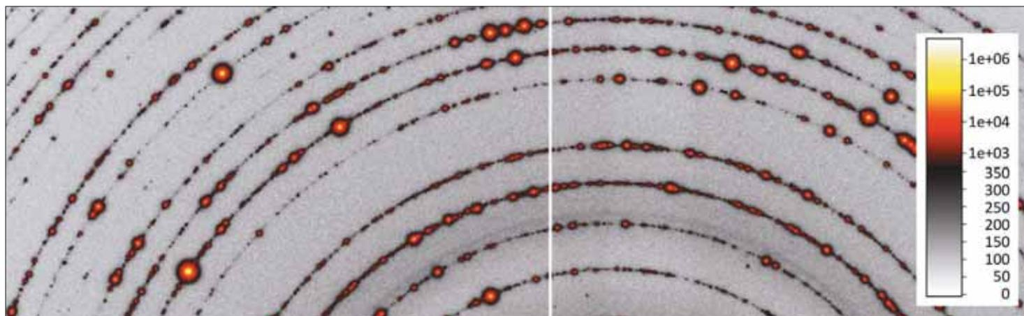
Powder data collected with an EIGER2 X CdTe system at the high-pressure beamline ID27, the sample containing large single crystallite species causing strong reflexes.
