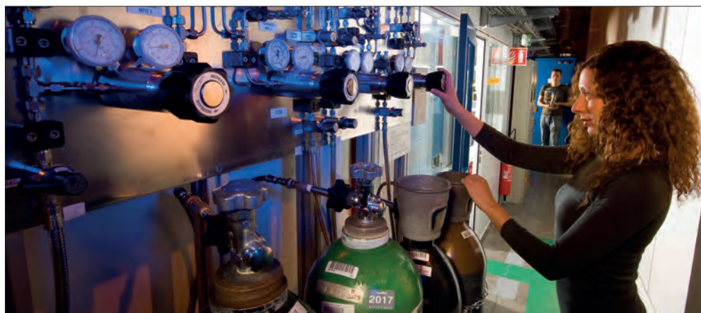
A state-of-the-art gas system allows catalysts to be studied under controlled flow, pressure and temperature.
