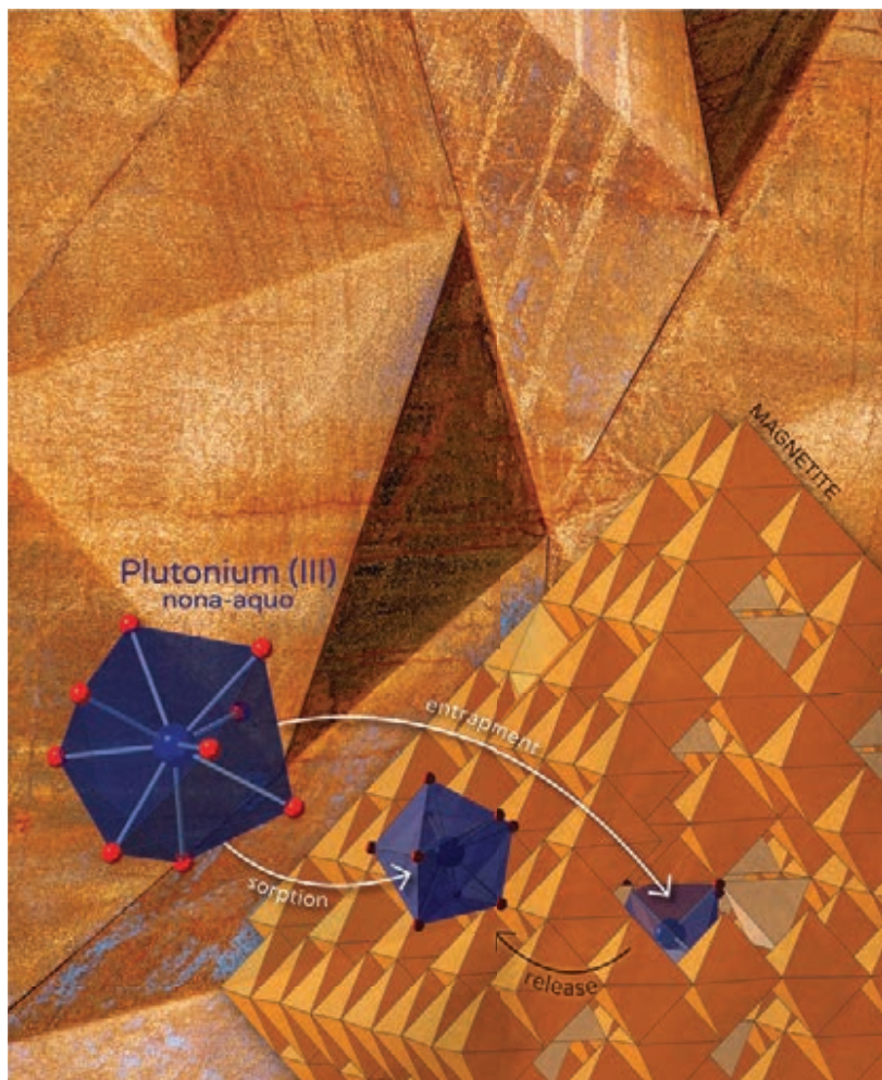
Fig. 128: Plutonium retention mechanisms by magnetite, a steel corrosion product, deciphered: structural incorporation proceeds through formation of pyrochlore-like islands, but recrystallisation of magnetite causes an expulsion of this structural plutonium, which is subsequently re-adsorbed at the most prevalent {111} faces constituting the surface of octahedral magnetite nanoparticles.
