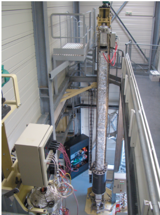
Fig. 147: NEG coating system for 6.2 m vacuum chambers.
