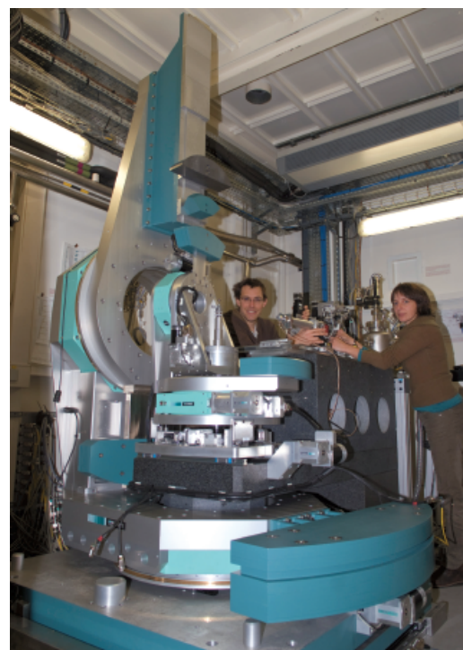
Fig. 3: T. Schulli and G. Carbone, scientists at beamline ID01 (UPBL1), with their new diffractometer for nanodiffraction analysis.
